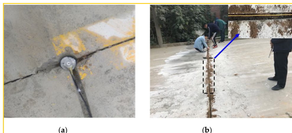
Figure 73. (a) Fiber Bragg Grating (FBG)-based acceleration sensor and (b) Distributed Optical Fiber Vibration Sensor [52].
